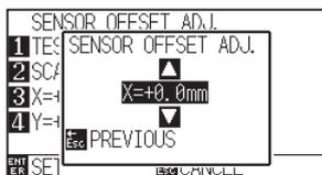
14 Press the POSITION (▲▼) keys and increase or decrease the setting value. Set the X value measured in step 12.
